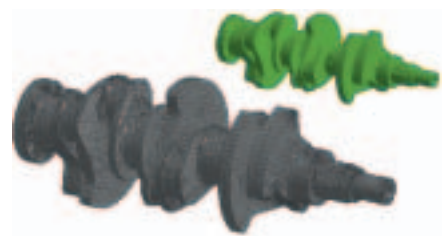
Hex dominant mesh of a crankshaft.
