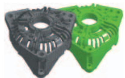
Hex dominant mesh of a machine cover.
